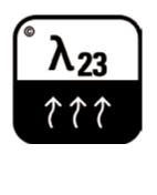
Thermal conductivity, extrapolated to  $23^{\circ}$  C
